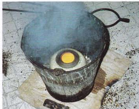
8 Pot withdrawn at 850°C and placed in container
