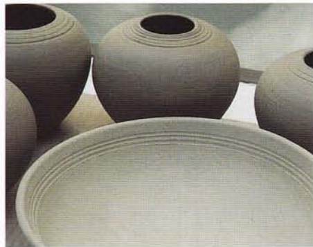
3 Work left to dry for biscuit firing to 1000°C
